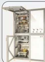
HKZ – High Pressure High Temperature Optical Floating Zone Furnace
